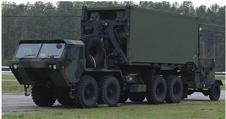
Figure 6. NGATS is a standalone test system contained and stored on two international standard 20-foot containers along with a 60-kilowatt generator. NGATS is a diagnostic test set used to troubleshoot LRUs in the field and is a mounted system that allows Army maintainers to fix-forward on the battlefield. (U.S. Army Acquisition Support Center photo)
