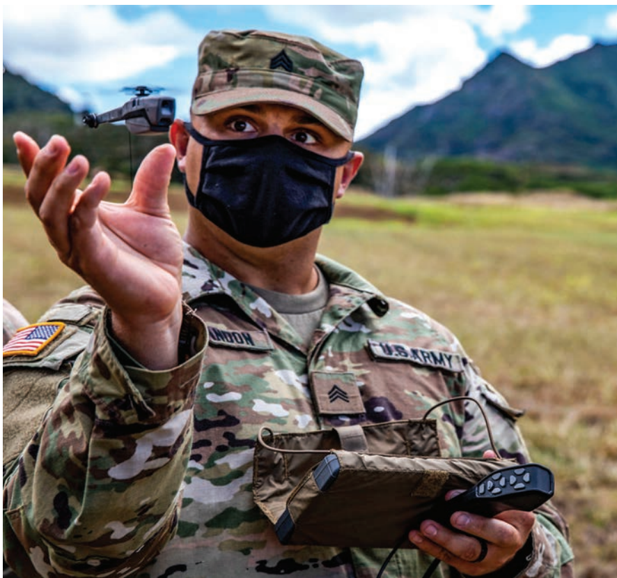
Figure 7. Soldiers train and certify on an SBS at Schofield Barracks, HI, Sept. 3, 2020. The sensor enables Soldiers to deploy a microdrone to gain situational awareness and observe where a Soldier cannot physically reconnoiter. (U.S. Army photo by SGT Thomas Calvert)
